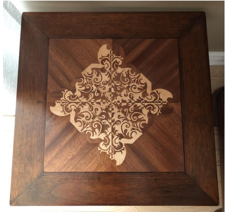
Finally finished my plant stand table! The pattern is my version of 17th French design in the Boule tradition in mahogany and maple. The 12" insert can pop out and be replaced with another insert changing the look of the table.
